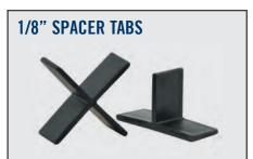
Hanover® can provide rubber-like Spacer Tabs for joint consistency. Not visible from the surface after installation is complete, spacers are placed between pavers to maintain 1/8" joints. See page 29 for more information.
