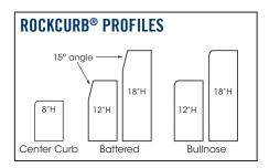
PLEASE NOTE: A range of Internal and External Radius sections are available. The 18" Radius Sections are produced with a Battered Edge or a Bullnose Edge. The 12" Radius Curbing is only produced with a Battered Edge profile and a limited number of outside radii.
