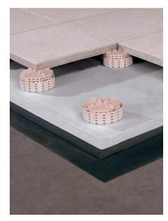
Using the Elevator®, High-Tab® or Standard Pedestal in conjunction with the Compensator® provides horizontal stability and joint alignment. Leveling Shims can be used for additional adjustments.
